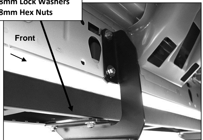
(Fig 11) Driver/left center Mounting Bracket installed
