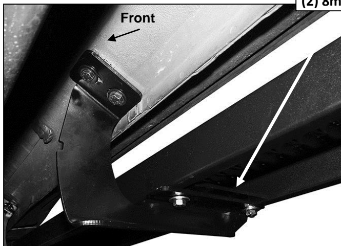
(Fig 12) Passenger/right center Bracket installed
