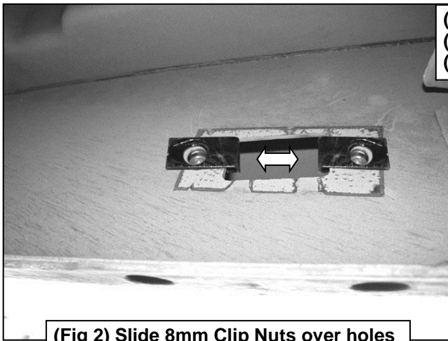
(Fig 2) Slide 8mm Clip Nuts over holes
