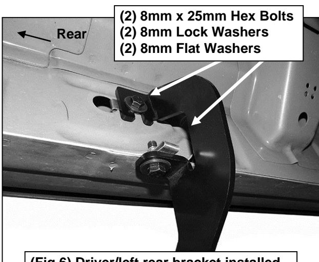
(Fig 6) Driver/left rear bracket installed
