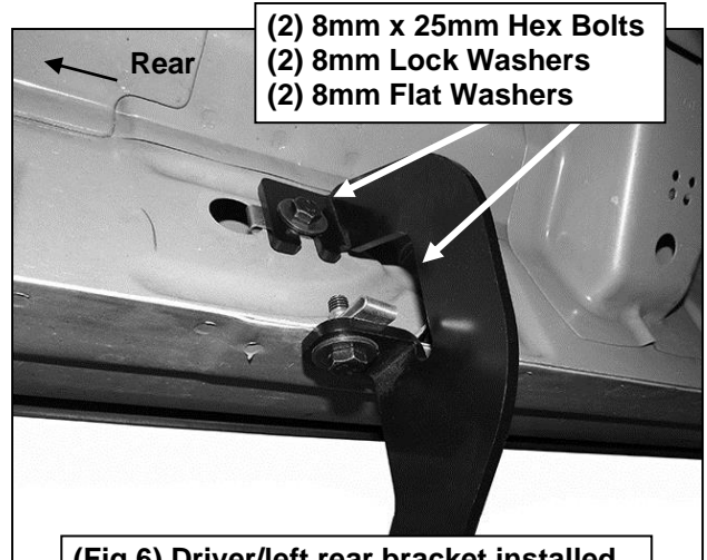
(Fig 6) Driver/left rear bracket installed
