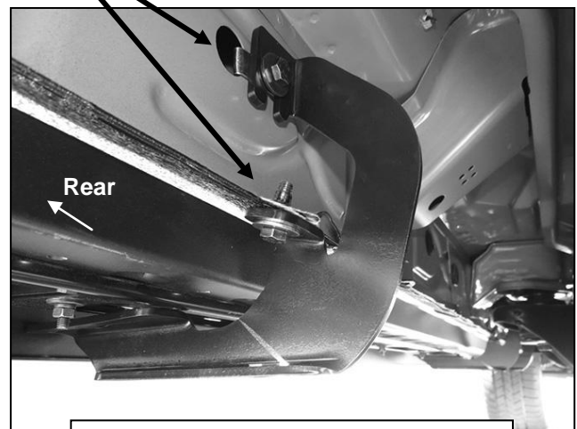
(Fig 10) Driver/left brackets installed
