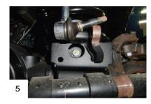
Remove lower shock mounting bolt located below spring.
