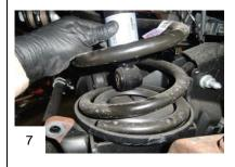
Slowly lower axle in order to remove shock and coil spring.
