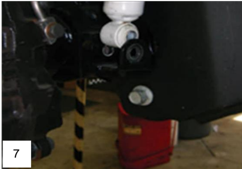
Disconnect door./pass. Front lower shock bolts.
