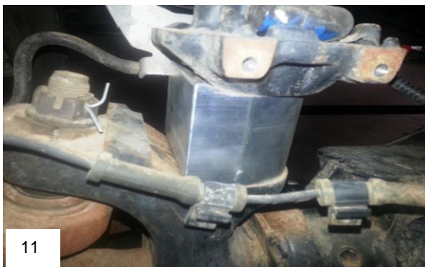
Place billet spacer on axle under spring perch. Secure with the provided hardware and torque to spec. Re-install the front spring and raise axle to hold in position.
