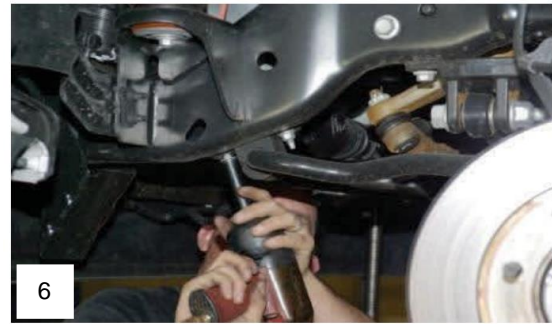
Remove factory sway bar bracket
