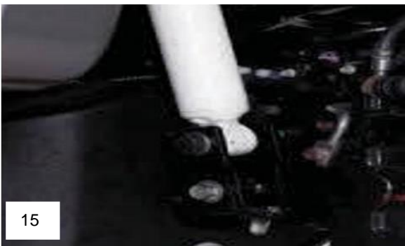
Install and tighten lower shock extension bracket
