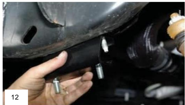
Install the sway bar drop bracket with factory hardware and torque to spec.
