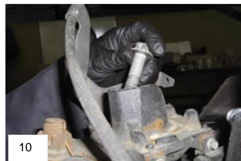
Remove bolt from middle of spring perch.
