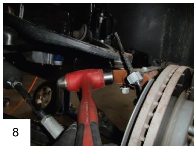
8 Carefully strike spindle as shown to separate ball joint.
