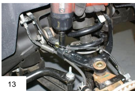
13 Reattach ABS/brake line bracket and sway bar end links.
