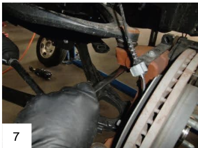
7 Loosen upper ball joint nut and leave attached.
