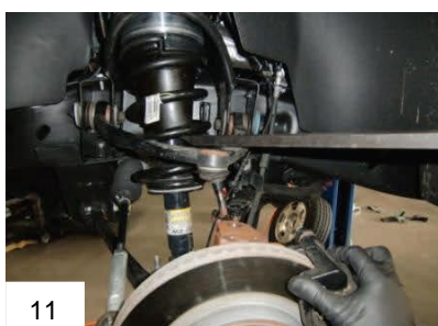
11 Lift suspension slightly while prying down to attach ball joint.
