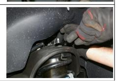
11. To remove the strut, lower it down through the control arm, then upwards and out over the spindle.
