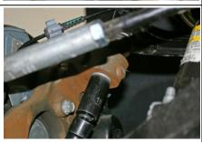
19. Return to the sway bar end link assembly and permanently tighten.
