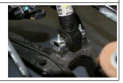
16. Once the lower strut mount is secured, return to the upper strut studs and permanently tighten all three nuts.
