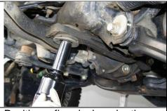
Position a floor jack under the front differential. Raise the pad so that it is touching the diff.
