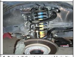
6. Reinstall the strut assembly in its stock location. Leave the three upper strut mounting nuts loose Raise the lower control arm and install the lower strut mounting bolt and nut. Use a floor jack to raise the lower control arm up in order to get the lower ball joint bolts installed. Be sure to use a thread locker on the lower ball joint bolts.
