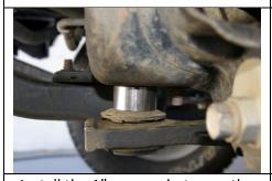
Install the 1" spacers between the differential supports and the front cross-member. Install the new bolts with factory washers and the new nuts and washers. Torque to factory specs.
