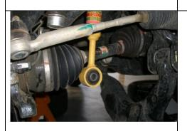
**4**. Remove the lower strut mount nut and bolt. Push the lower control arm down.
