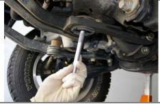
Remove the factory 19mm differential mounting nuts and bolts. The OEM washers will be reused.
