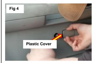
6. Remove the plastic cover inside the door handle. Insert the flat head screw driver behind the plastic cover and pop it off. See figure 5.
