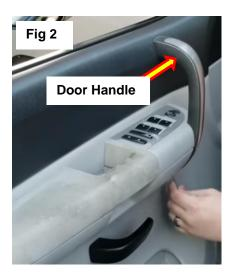
4. Remove the door handle by pulling the pin in the door handle down using a flat head screw driver. See figure 3.
