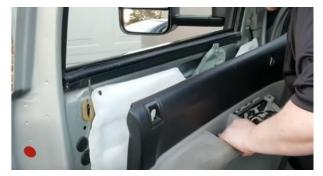
10. Remove the piece of foam by hand to reveal the three 10mm nuts which are used to hold the mirror to the door. See figure 6.
