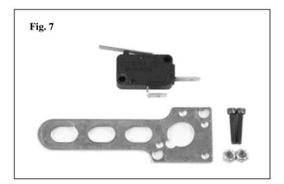
**C.** The throttle switch bracket is made of easily formed material. Attach the end of the bracket to one of the throttle body studs and bend the bracket in such a way to allow the throttle arm to contact and depress the switch's lever at wide open throttle.
